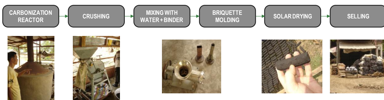
Figure 17 – Charcoal “briquettes” fabrication process, Source: ENEA Consulting, adapted from GERES, 2006
