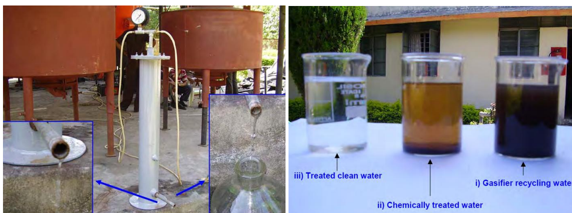
Figure 23 – Water treatment plant and water quality along the process, Source: Ankur Scientific
