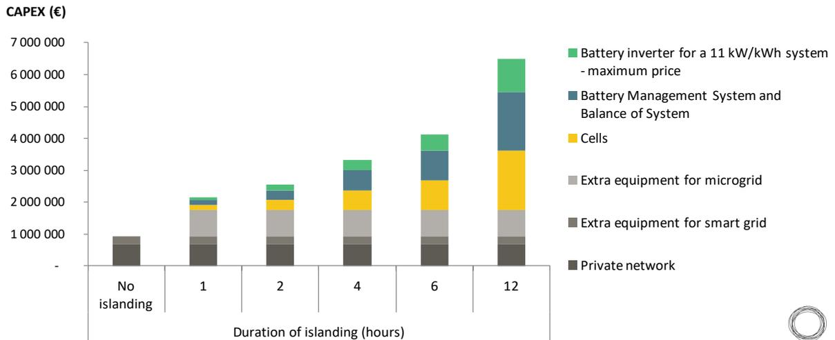
Figure 21 – CAPEX of equipment needed for the islanding function<sup>50</sup> depending on the required islanding time (Enea Consulting analysis based on [32, 33, 19, 34, 35, 36, 37] for grid equipment and [38, 39, 40, 41, 42] for batteries)
