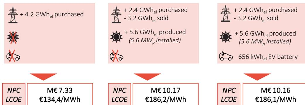
Figure 9 - Comparison of grid-only scenario with local generation scenarios (local generation only, use of vehicle-to-grid system, and use of a grid-scale battery)<sup>23</sup>
