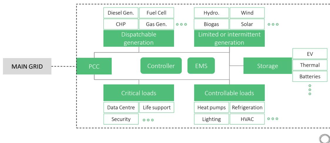
Figure 2 - General representation of a grid-connected microgrid<sup>11</sup>
