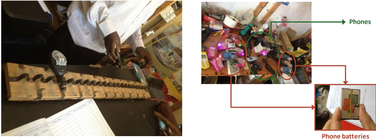
Figure 17 -- Environment challenges to plug-and-play kits: Homemade socket and battery charging instead of phone (Source: ENEA Consulting field investigations, 2013 )
