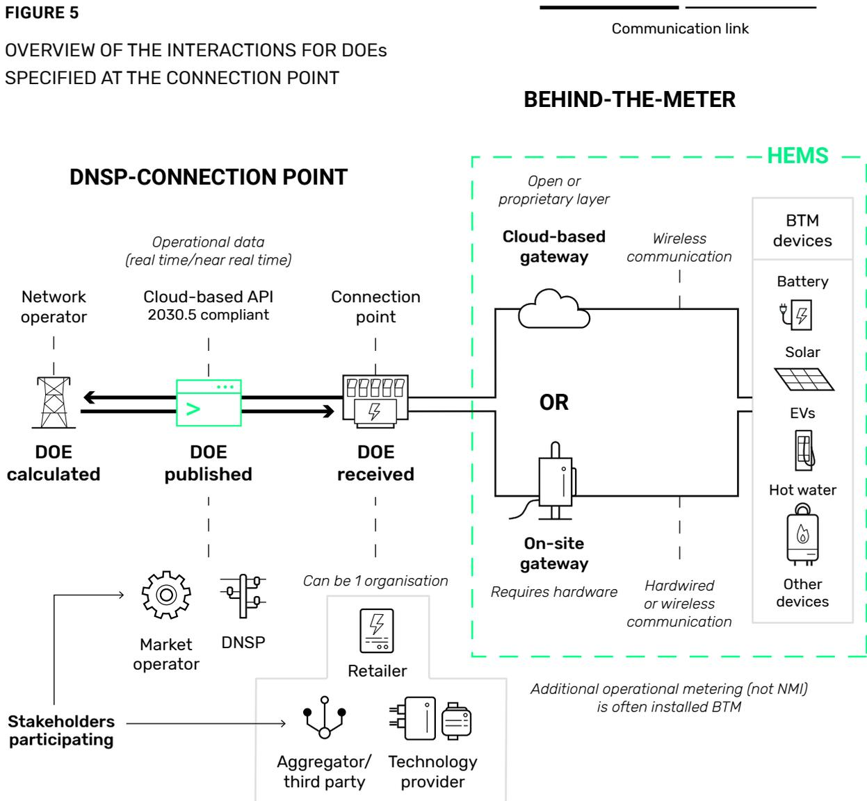
For DOEs specified at the customer connection point, the total behind-the-meter power flows will need to remain within the published limits. In the near term, it is expected that a single device (for example a solar PV system through a smart solar
