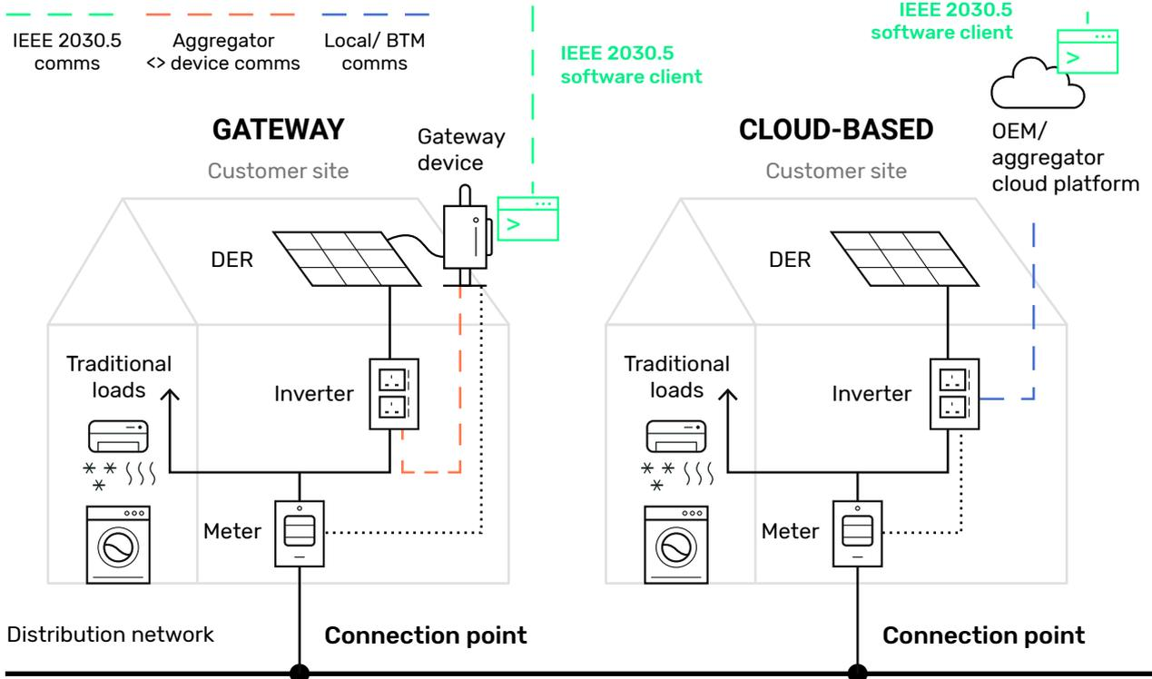
Although it is the smart inverter receiving and acting on the DOE, the power flows of the entire site still need to be considered.
