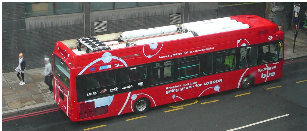
Figure 10: The six roof-mounted hydrogen fuel tanks of a London fuel cell bus
