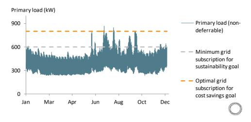
Figure 8 – Relevant grid subscription choices with respect to non-deferrable load profile
