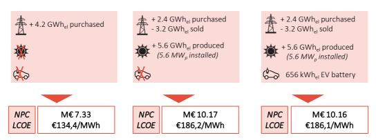
Figure 9 - Comparison of grid-only scenario with local generation scenarios (local generation only, use of vehicle-to-grid system, and use of a grid-scale battery) <sup>23</sup>
