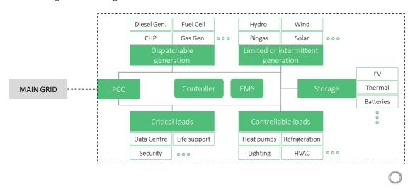
Figure 2 - General representation of a grid-connected microgrid<sup>11</sup>
